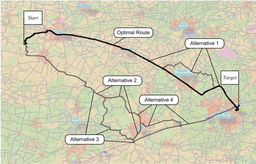
Fig. 4 Example computation of alternative routes (opt. route length = 35 km;  $\nu = 1.1$ ;  $\ell = 5000$  m)
